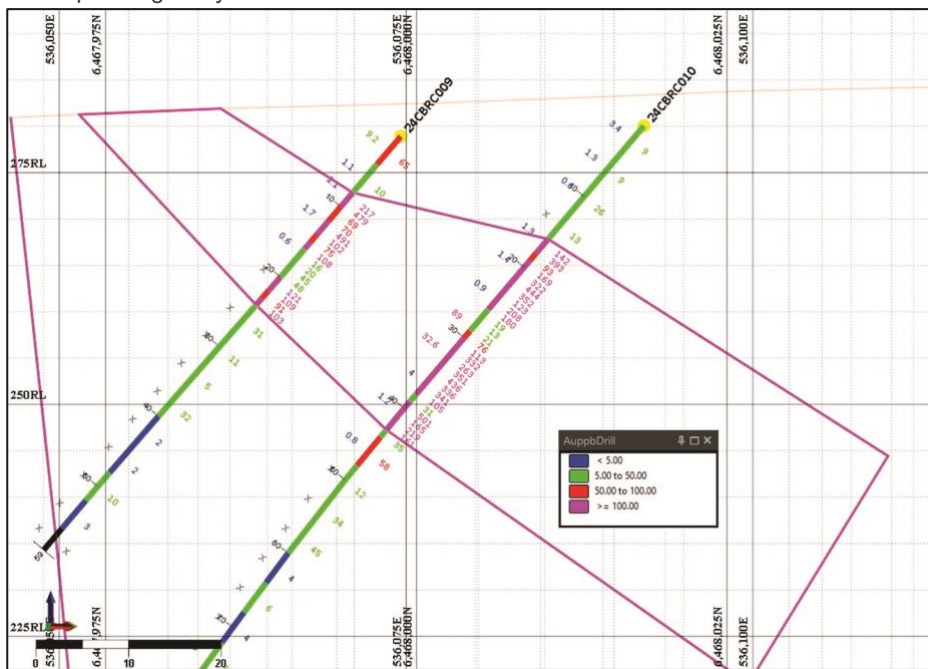
Figure 2: Cubbine Section 6468005N (Northernmost section) with Au ppb on the right and As ppm on the left. Pink outline on the left is the granite contact and the pink envelope shows the interpreted gold system.
